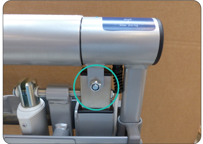
Dismount the bar from the actuator fitting
