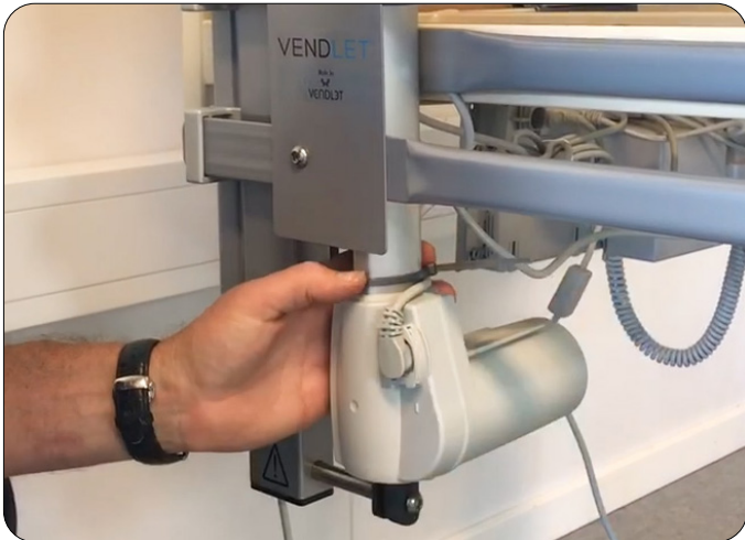
Place the actuator cable behind the actuator with cable ties
