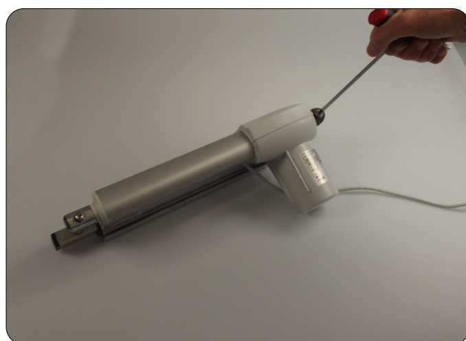
Remove the Allen screws and free the actuator
